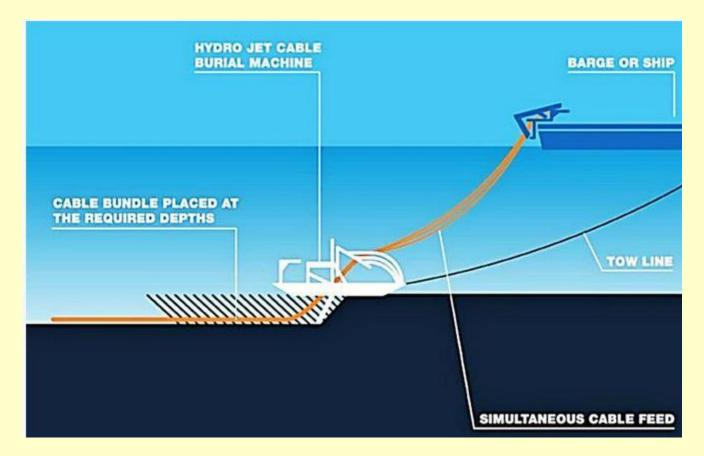
The work is done with the help of acoustic instruments such as **echo-sounders and accurate Global Positioning System (GPS) and differential GPS**. The ROVs dig the trench in which the transmission cable is laid fix the cable on the right route and cover the cable with sediment. Burying the cable in the seabed is a slowly and costly operation but it is paid back by its reliability and extended lifetime.
